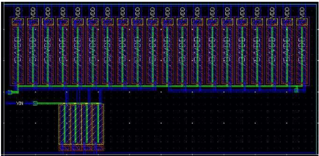
Figure – 3.10: Layout for Common Source Amplifier with PMOS Current Mirror Load
