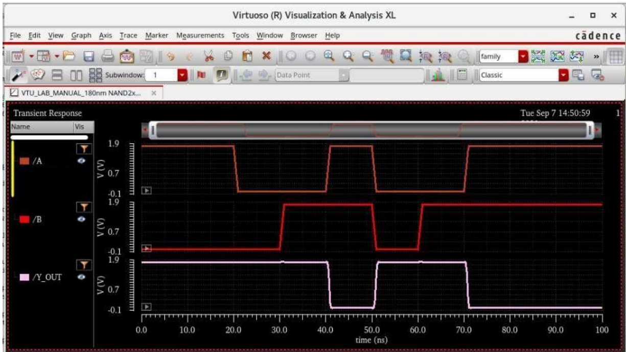
Figure – 2.9: Transient Analysis of 2 – input CMOS NAND Gate
