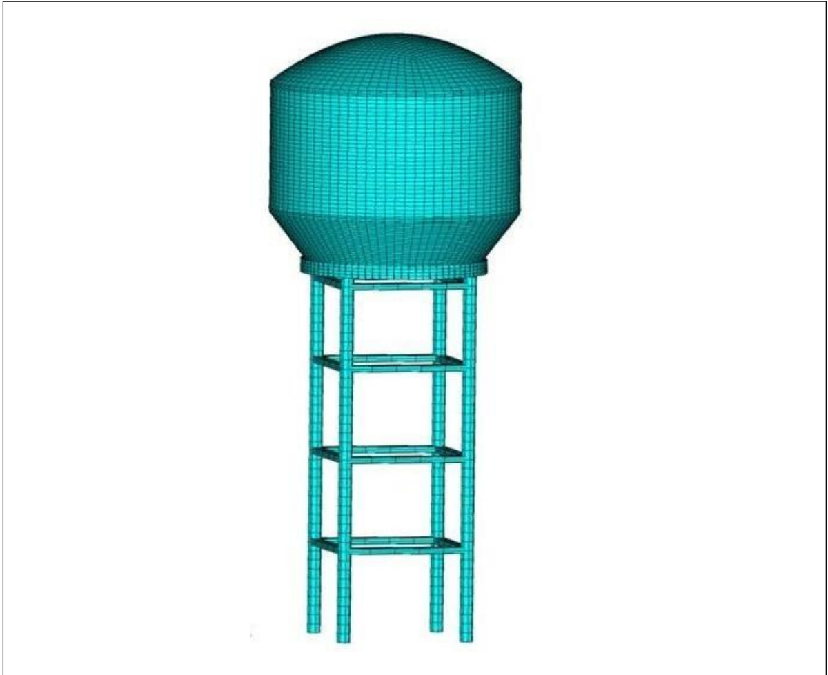
Fig.13. Circular water tank
