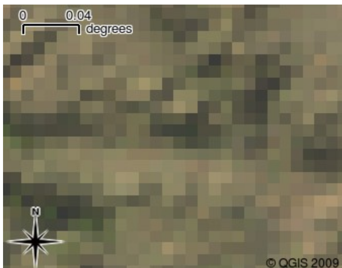
Fig. 2.22 The same raster data, but this time zoomed in. The grid nature of the data can be seen.
