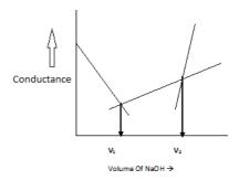
Where,  $V_1$ = Volume of NaOH required to neutralize HCl. ( $V_2$ - $V_1$ ) = Volume of NaOH required to neutralize acetic acid.
