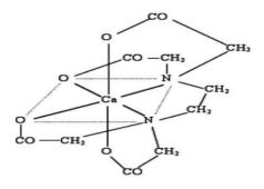
When the solution is titrated with EDTA, EDTA combines with the free metal ions (calcium ions in preference to magnesium ions) present in the solution. At the end point, when all the free metal ions are exhausted, added EDTA dissociates the wine red cold metal-EBT complex, consumes the metal ion and releases the blue cold free indicator. Hence the color changes from red wine to blue.
