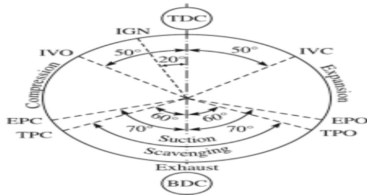
Figure : Port Timing Diagram of A Two Stroke Petrol Engine.
